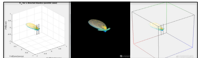
Figure 2: Phased-Array Antenna Beam Pattern Created in Matlab .m Source and Converted to .x3d and .wrl Models.
